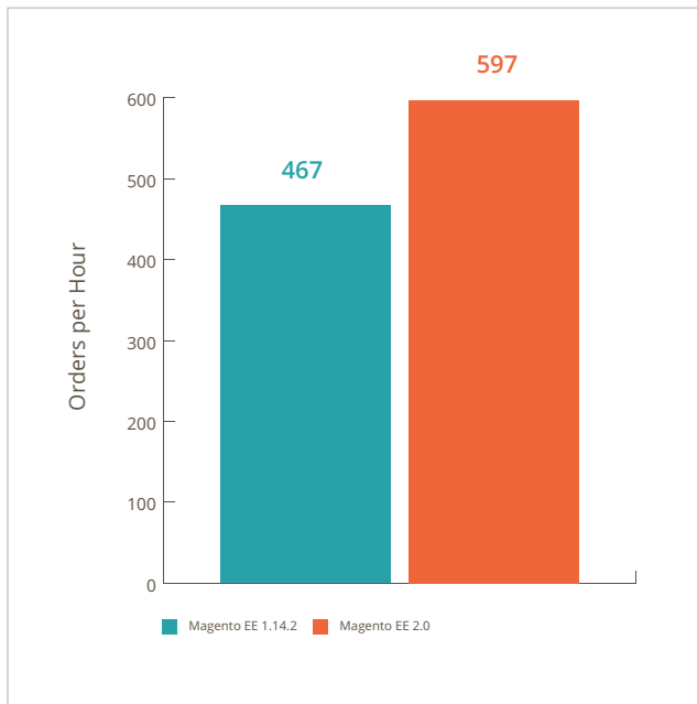
FIGURE 4: Throughput results for 25 JMeter threads show that Magento Enterprise Edition 2.0 can process 597 orders per hour, which is 28% more orders per hour than Magento Enterprise Edition 1.14.2.
